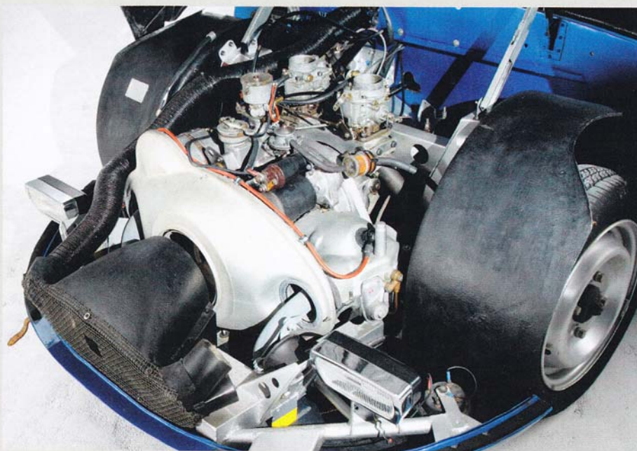
Left: just room for a little finger in filler-flap hole. Below: 848cc flat-twin fed by twin Solexes; Sferma blower gave it equivalent capacity for sub-1200s
